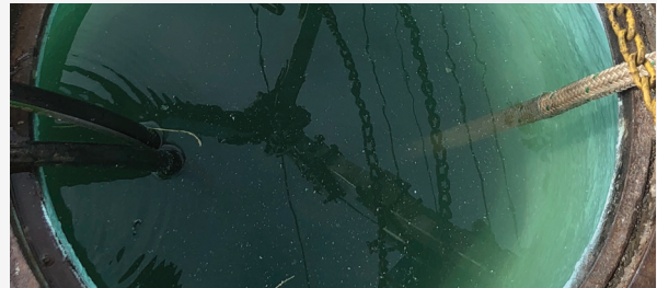
Lined manhole is filled with water for leak (exfiltration) testing. No leaks present.
