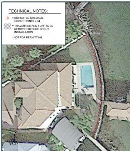
*Injection port, to install I & I Guard-SSF, identified along condo property seawall, will fill voids caused by erosion and prevent seawall from collapse.*
