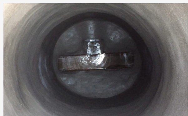
GeoKrete Geopolymer showed no signs of cracking and peeling.
