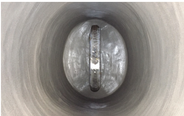
GeoKrete Geopolymer showed no signs of cracking and peeling.
