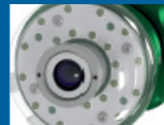
CCD camera with LED illumination
